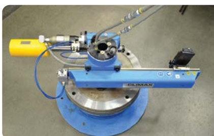
FF6300 299.7 - 1524.0mm Facing diameter Pneumatic or hydraulic
