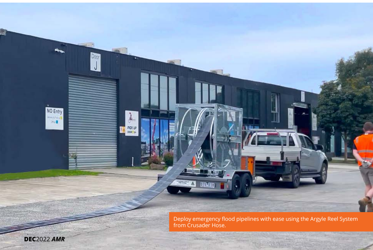
The Crusader Hose Rapid In-pit Dewatering System features the Hamersley™ Reel System and Waterlord® layflat hose.
