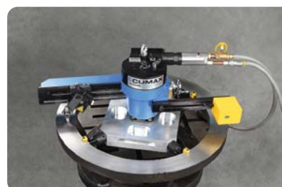
FF5300 144.8 - 1016.0mm Facing diameter Pneumatic
