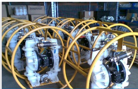
The Sandpiper range of plastic-bodies flap-check valve pumps are ideal pumps for mine dewatering applications: one that is lightweight, resistant to corrosion, easy to maintain and able to pass large solids.
