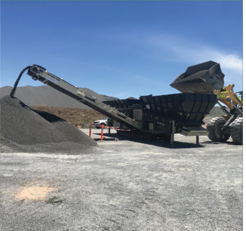
IMS – BP1200-9TB Track Blender with two 5.5 meter long feed hoppers with mixer and production up to 1000 tonnes per hour.
