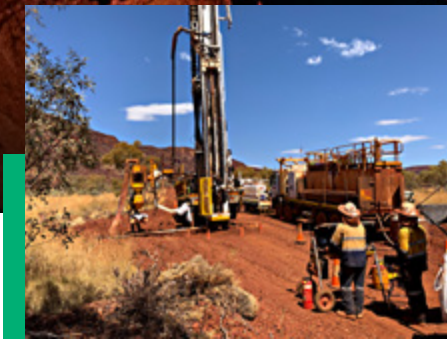
A REVERSE CIRCULATION RIG BEING OPERATED BY MINING DRILLER FORACO. A REMOTE OPERATOR CONTROL PANEL IMPROVES SAFETY BY POSITIONING THE DRILLER FURTHER AWAY FROM RIG.
