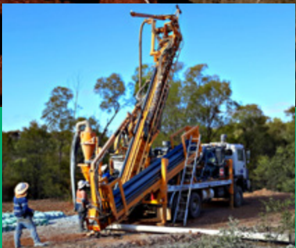
A REVERSE CIRCULATION RIG OPERATED BY EAGLE DRILLING IN NORTH QUEENSLAND.
