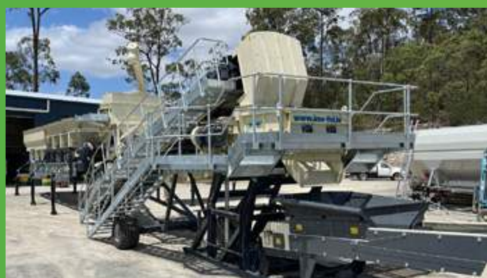
IMS electric modular Pugmill & twin hopper Blender with and 24-meter radial conveyor with auto radial return and auto lift as the stockpile height increases, fully automated and in stock. Option of four hoppers.
