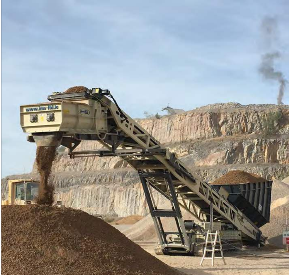
IMS – PM1050-16TB Track Pugmill with adding Powder and liquids options, fully automated with production of up to 500 tonnes per hour.
