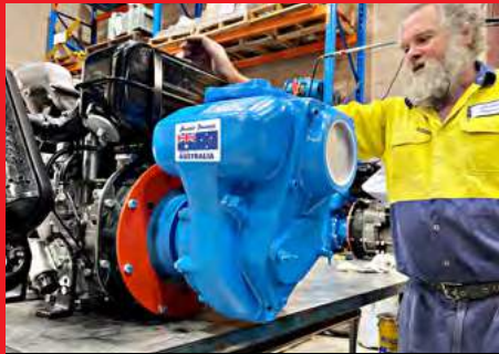
In production, the 4" B4XR-A/ST being fitted to the Kohler KD625 engine.
