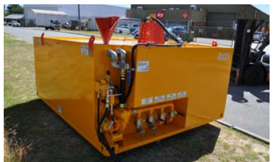
Fresh off the production line, a mud tank fitted with an Aussie GMP hydraulic drive pump.
