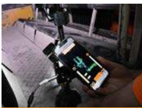
GeoSLAM Revo RT (Real Time) System showing the captured point cloud live on a phone in 3D during scanning to make sure all required areas are captured.
