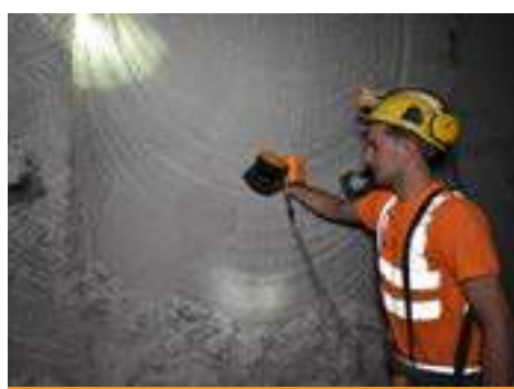
Georeferencing using adjust to control with the GeoSLAM Horizon, automatically capturing the control point sideways which will have the offset automatically calculated.
