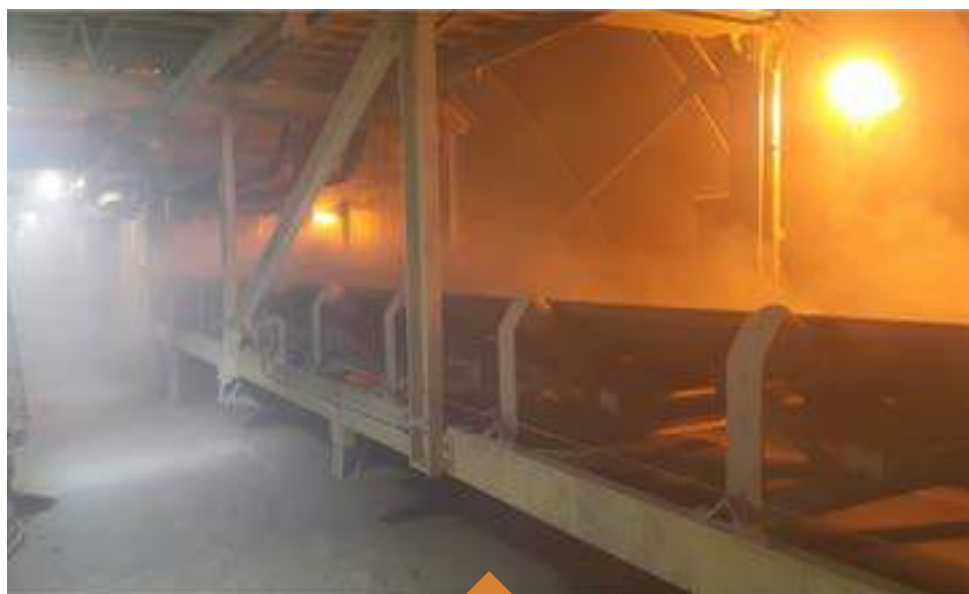
Dry Fog settles out dust down to respirable levels without adding moisture.
