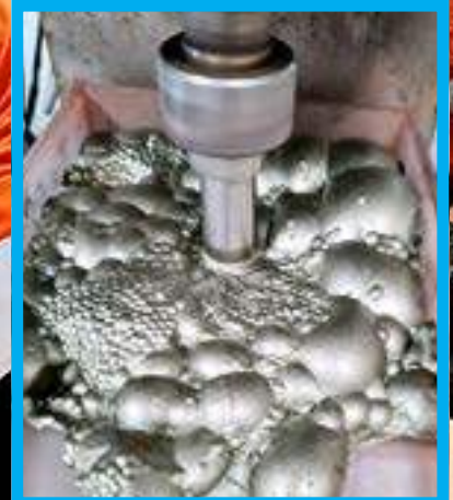
Froth flotation carried out by InterChem. It is a highly versatile method for physically separating particles based on differences in the ability of air bubbles to selectively adhere to specific mineral surfaces in a mineral/water slurry. The mineralised froth obtained in the image shown is typical of copper ore types processed in South Australia. InterChem Mining is looking forward to supporting clients and new customers with site specific laboratory screening and plant-based trial work.
