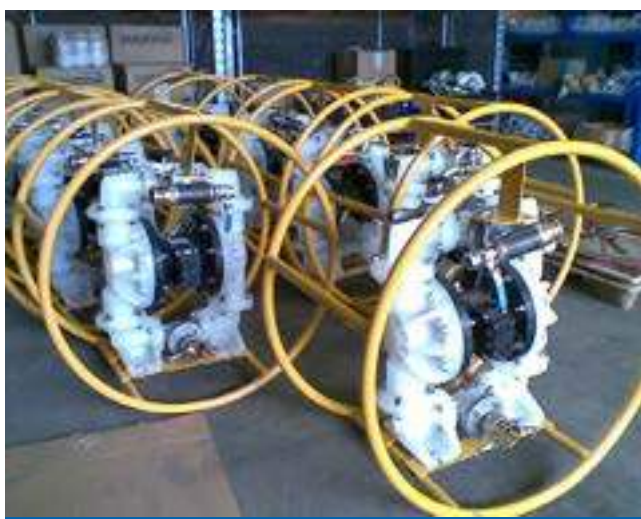
The Sandpiper range of plastic-bodies (non-metallic) flap-check valve pumps are ideal pumps for mine dewatering applications: one that is lightweight, resistant to corrosion, easy to maintain and able to pass large solids through the system.
