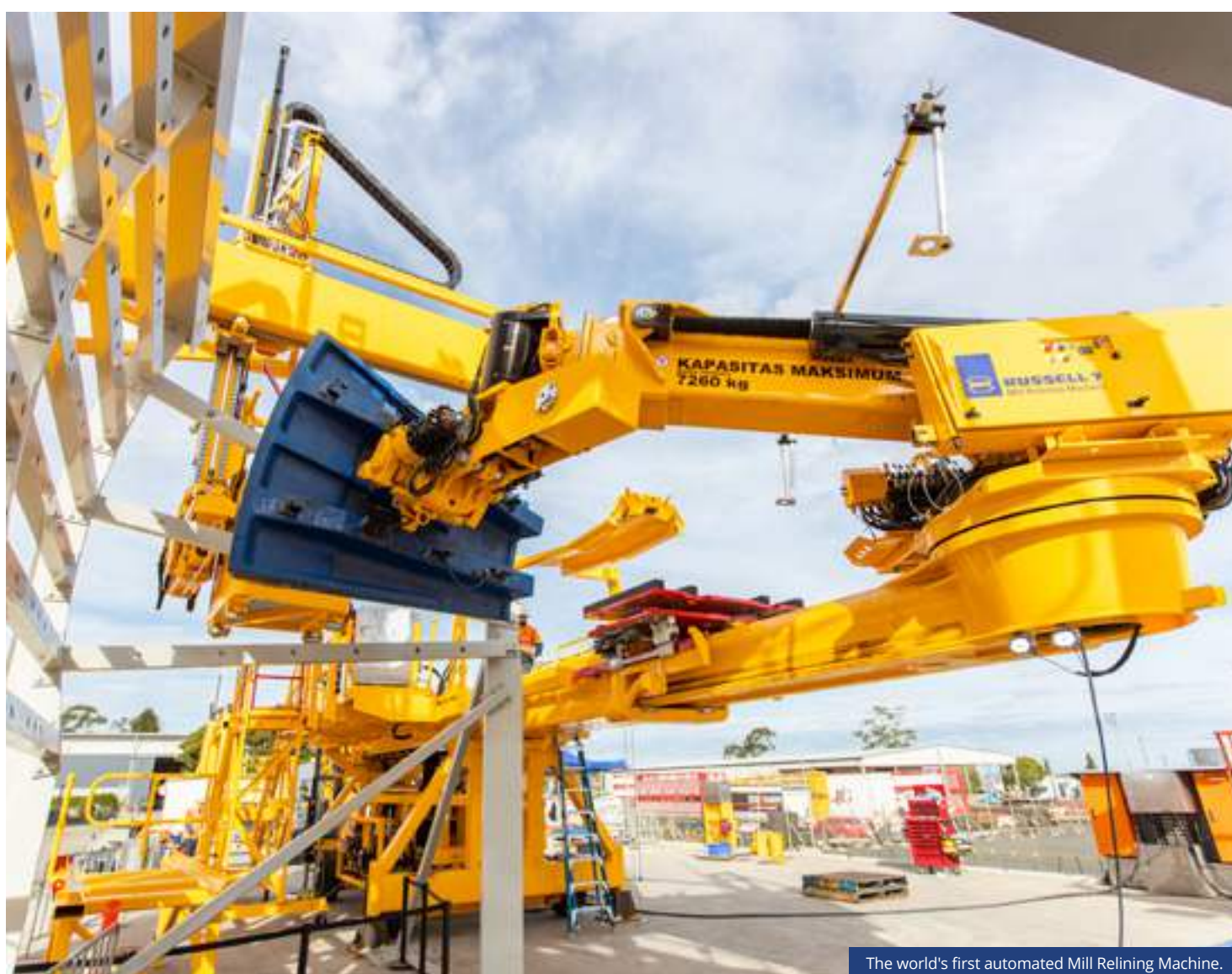
Factory commissioning of RME's first automated mill relining system THUNDERBOLT SKYWAY project.
