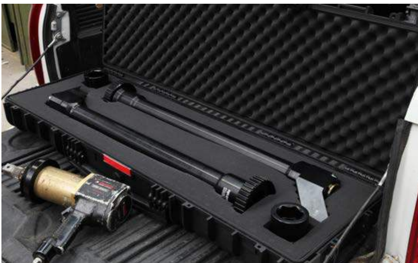
The Lightening Bolt tools have been designed to replace heavy extension tools currently being widely used the world over for aiding in the removal of heavy vehicle wheel nuts.
