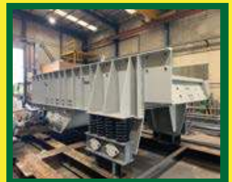
HAWK Extra Heavy Duty Mining Standard Vibrating Feeder under the dump hopper to handle 1000 TPH of minus 1000mm rock
