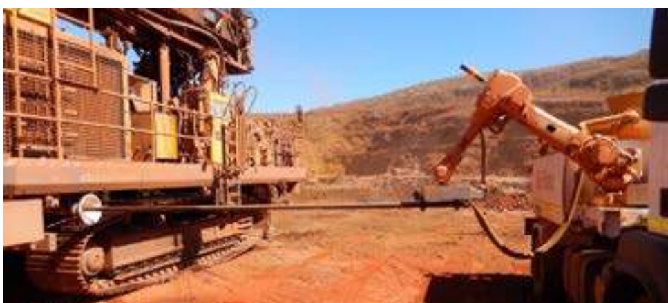
The robotic Mobile Fluid Transfer System can be fitted to a standard water truck and automatically transfers the water.
