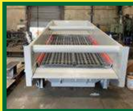
HAWK Extra Heavy Duty Mining Standard Horizontal Scalping Screen to handle 900 TPH of rock
