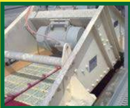
Hi-Flow Dewatering Horizontal Screens
